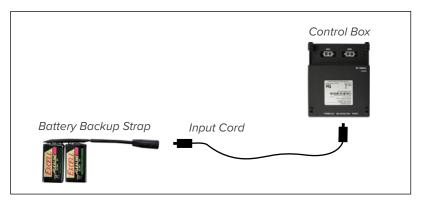
**Note:** Detach the Battery Backup Strap after the emergency is over, as the system will continue to draw power from the batteries even if not in use.
